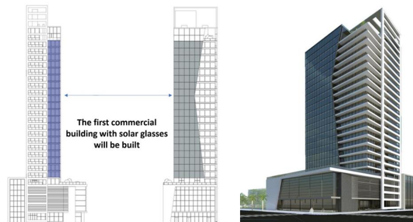
AMB Brasil’s artists impression of ‘Imperiale’ building including anticipated deployment of ClearVue PV IGUs to façade.
