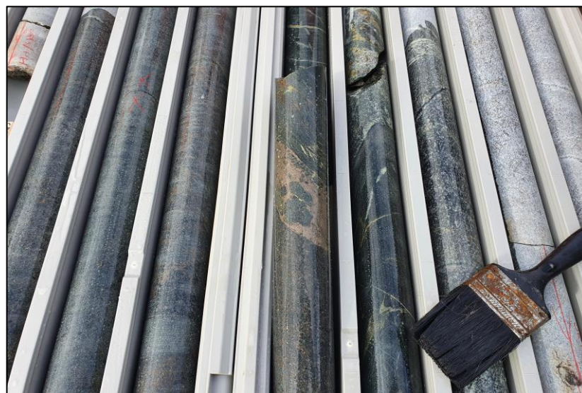
Figure 1. Anomalous Ni-Cu-PGE bearing sulphides in diamond drill hole CBDD028 at the T5 Ni-Cu discovery zone (161m-169m shown).
