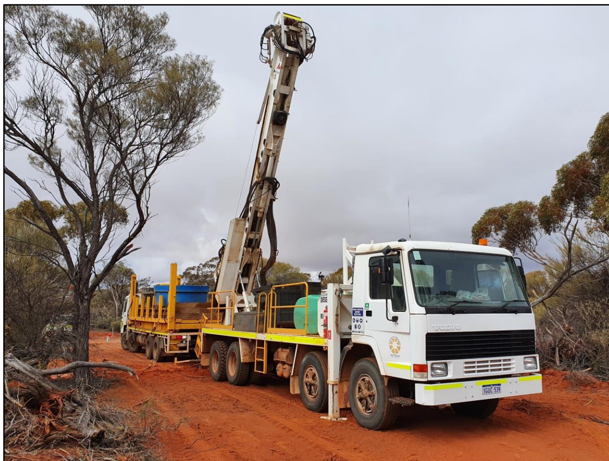
Figure 2. Topdrive Drillers Australia diamond drill rig and rod carrying service truck over CBDD028 collar location Target 5 prospect area Carr Boyd Nickel Project
