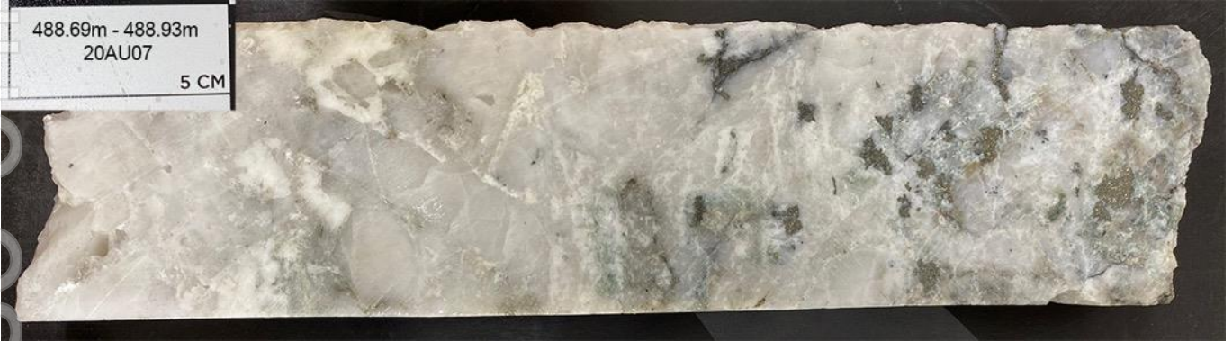
Figure 2 Hole #7 (20AU07) 488.69m - 488.93m quartz vein with arsenopyrite, pyrite and pyrrhotite.
