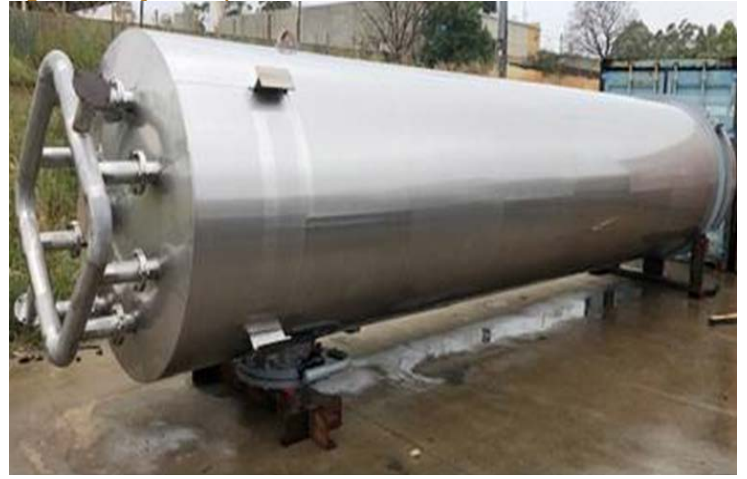
Figure Twenty Seven | Six Tonne Elution Column
