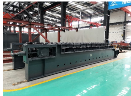
Figure Twenty Five | Apron Feeder
