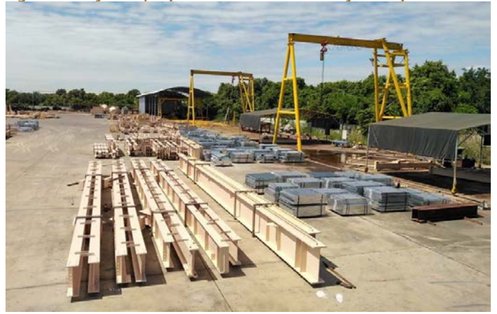
Figure Twenty Nine | Top of Tank Steel Work ready for shipment to site
