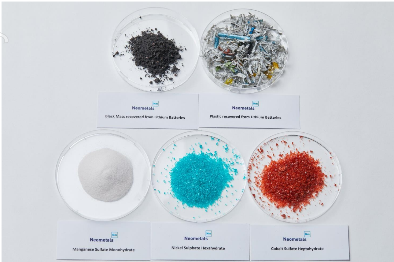
Figure 5 – Sample of products generated using the Primobius LIB Recycling Technology
