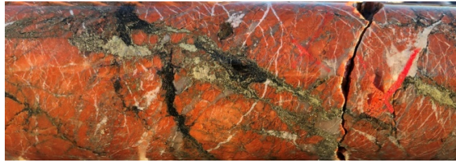
Figure 15. Chalcopyrite and pyrite fracture infill hosted by a mylonitised Pegmatite – HTODD001, 212.6m.
