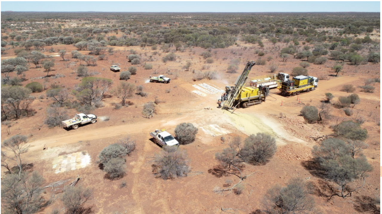
Figure 1. Reverse Circulation Drilling underway at Target 1
