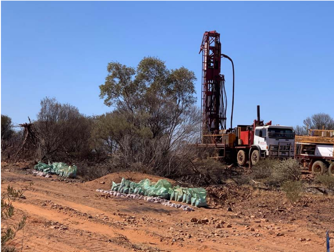
Figure 7: RC drill rig at Wiluna West C4 Iron Ore project completing grade control
