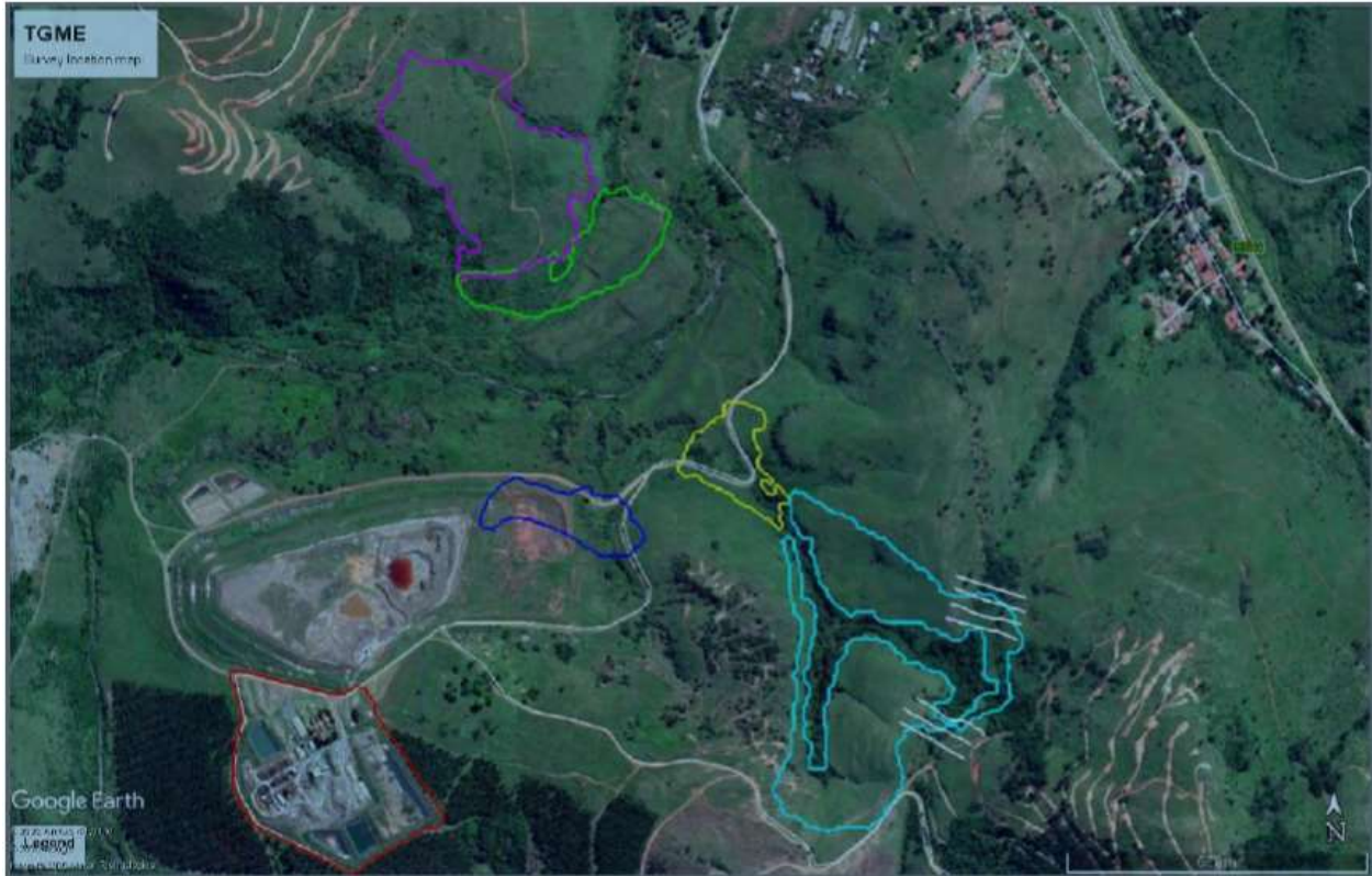
Figure 3: Location map of TGME gravity surveys. Plant (red), Balancing PCD (blue), Wishbone SW Dam & FSL (yellow), IOTA PCD (green), Wasterock N (purple), Wasterock S (cyan) & fault lines (white)
