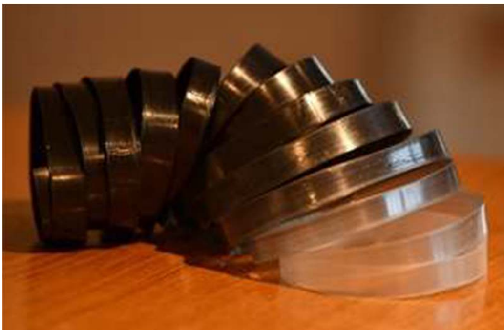
Figure 1. EdenPlast®- carbon nanotube infused polymer
