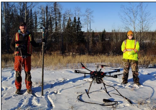
Figure 5- UAV Magnetic Survey Equipment Setup at South Limb
