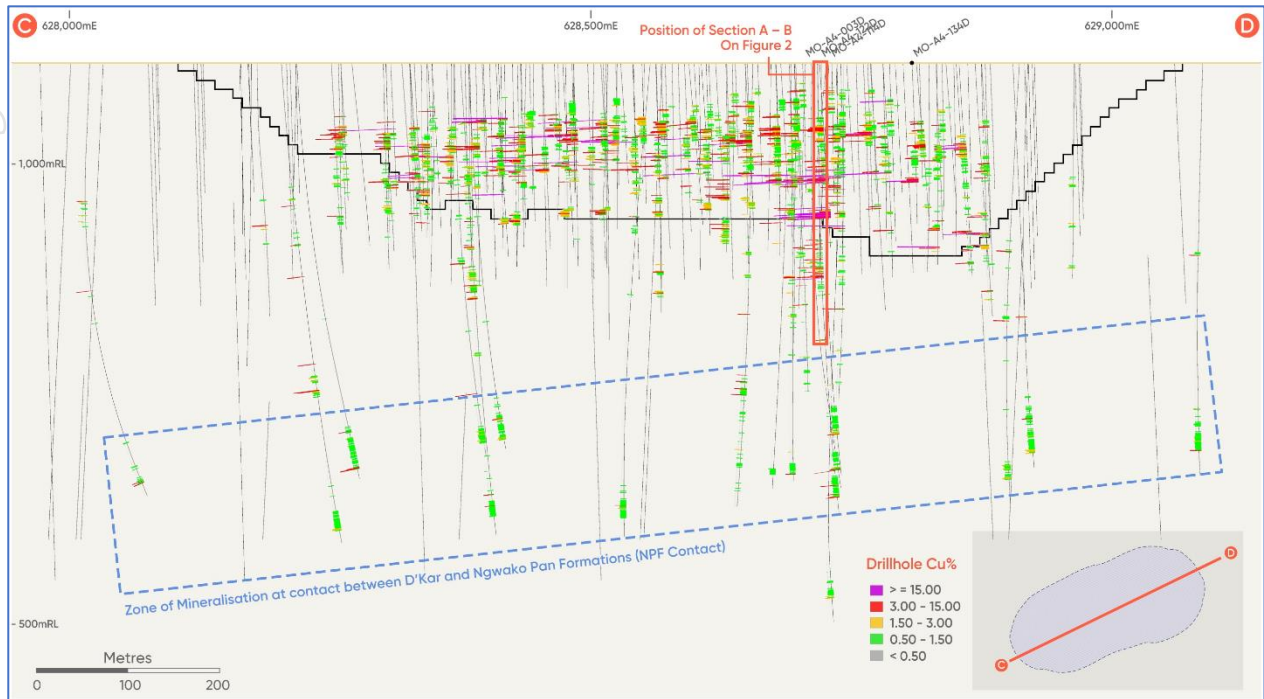
Figure 3: A4 Longitudinal projection looking north showing optimised pit shell for the A4 Maiden Resource and copper grades represented as histograms for holes where assays have been received. Deeper intersections within the blue rectangle are related to NPF contact mineralisation announced previously by MOD Resources.
