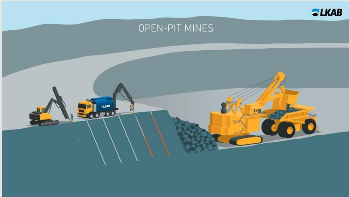
Figure 8.2 Waste drilling with face shovels and trucks
