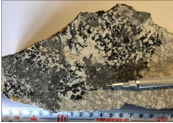
Figure 3.6 Clusters of high grade disseminated coarse wolframite showing haloes of coarse arsenopyrite. This sample returned 16% WO 3 .
