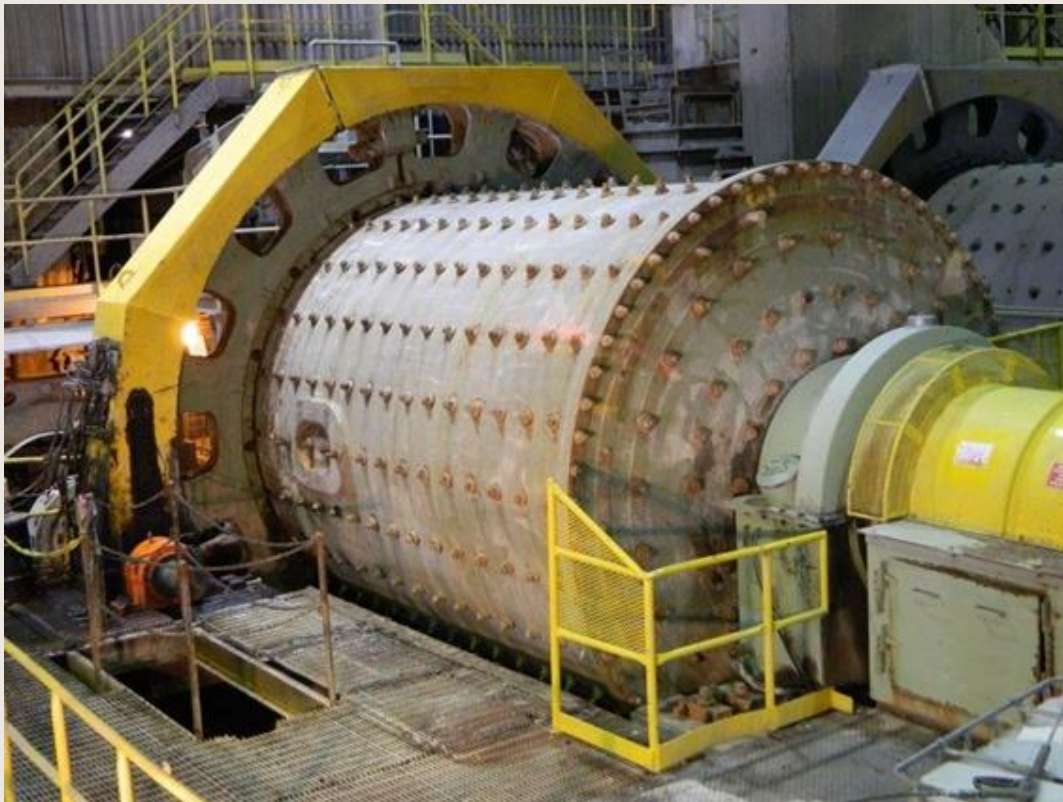
Figure 9.5 Grinding section - a used Allis Chalmers 3.8m x 4.6m 1100kW Rod Mill
