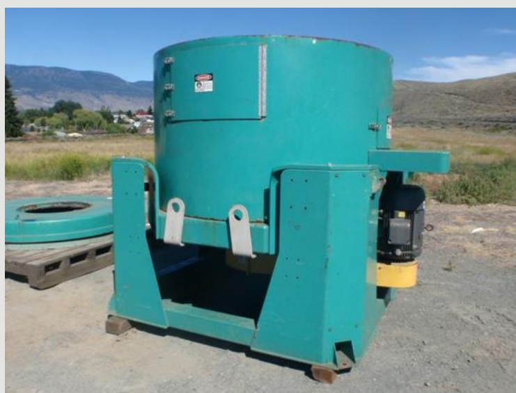
Knelson 48 CVD Hi-G centrifugal concentrator
