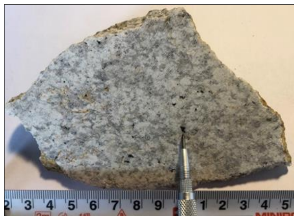
Figure 3.5 Disseminated millimetric crystals of wolframite hosted in endogranite. This sample returned 0.46% W.
