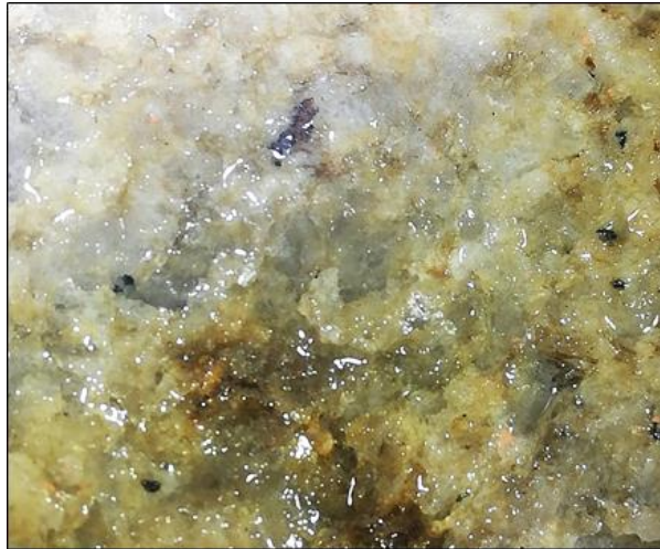
Figure 4.1 Image from COPAREX underground workings at Mina Carmen. The dark disseminated spots consist of millimetre crystals of wolframite hosted in the endogranite.
