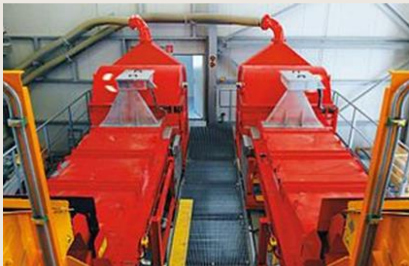
Figure 9.2 TOMRA X-Ray sorting equipment Twin XRT 1200 sorting units
