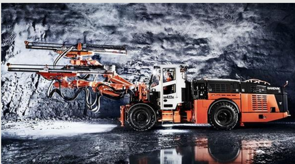
Figure 8.3 Underground development drilling Twin boom development jumbo
