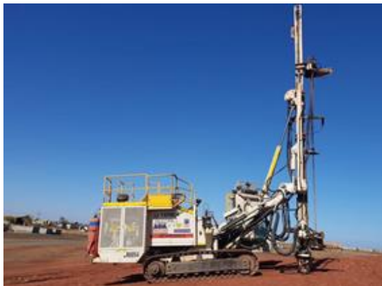
Surface blasthole drill and sampling rig
