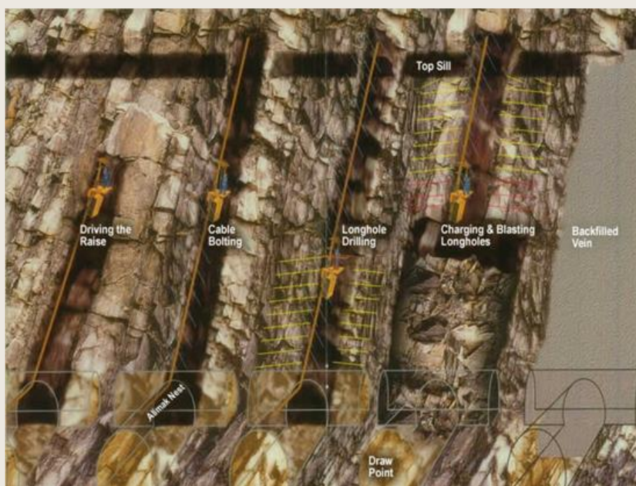
Figure 7.1 Modern raise mining methods Schematic of raise mining progression
