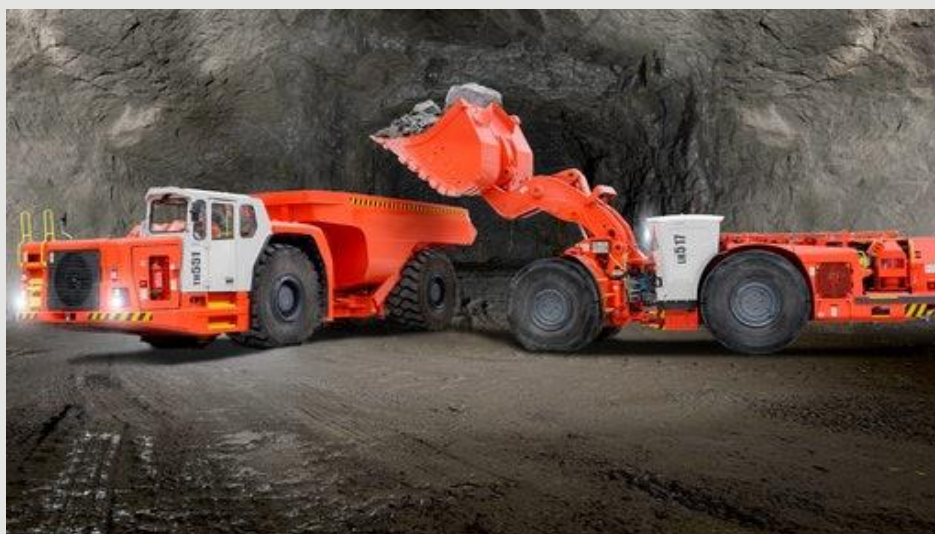
Figure 7.2 Underground mining equipment LHD loading dump trucks underground
