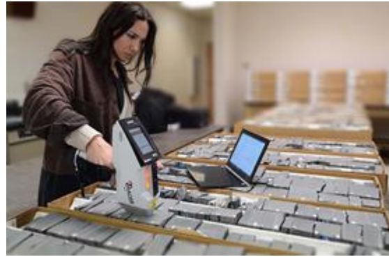
Use of a handheld X-Ray fluorescence analyser
