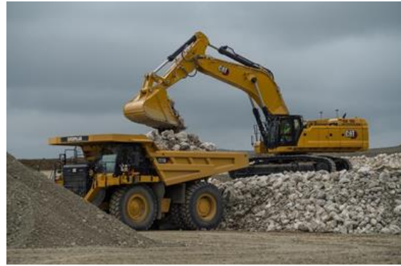
Figure 6.7 Backhoe excavator loading ore into dump trucks on 4m benches
