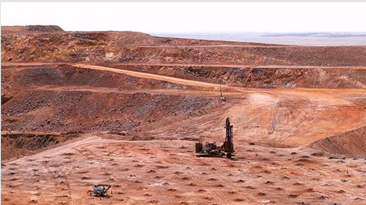
Figure 8.1 Waste drill pattern for large scale blasts
