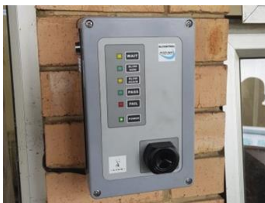
Figure 14.1 Mine site breathalyser. Mine entrance breathalyser for alcohol & drug screening prior to working on site.
