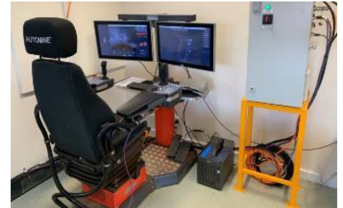
Recently installed tele-remote loader operating station at surface in Leonora
