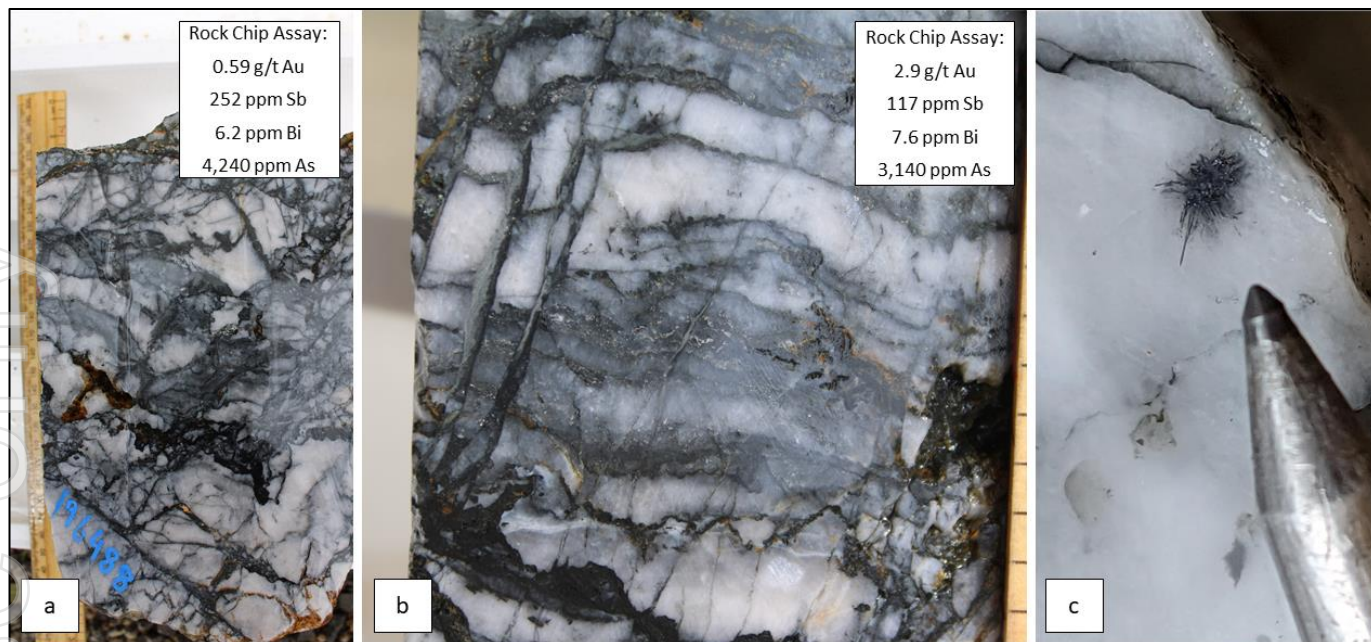
Figure 5: Rock samples collected from the Fentiman's South historic mine waste dump (scale ruler in cm): (a) mineralised quartz vein with abundant stylonite and breccia textures; (b) disseminated sulphides (arsenopyrite, stibnite and pyrite) within a stylonitic and brecciated quartz vein; and (c) coarse stibnite ( \text{Sb}_2\text{S}_3 ) crystals and thin stylonites within a mineralised quartz vein
