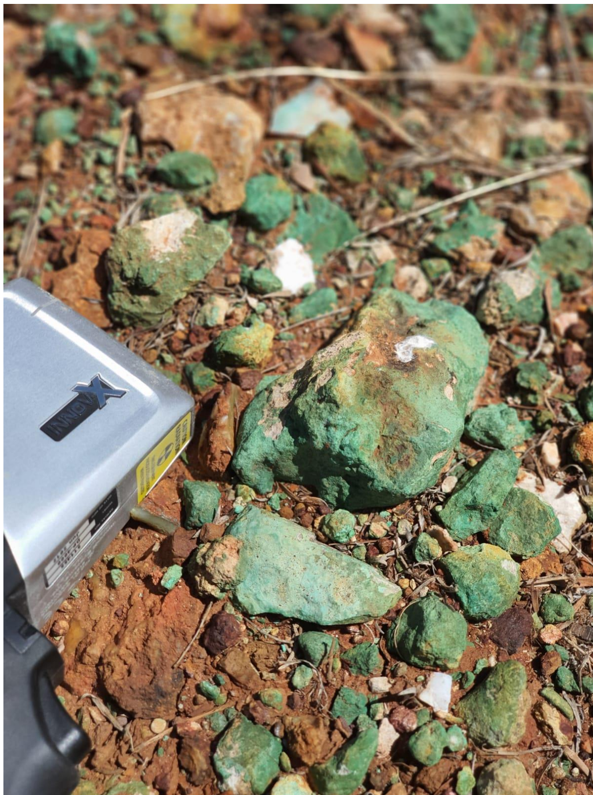
Figure 2 Crosswinds Copper Prospect - Malachite (copper carbonate) mineralisation exposed in table drain
