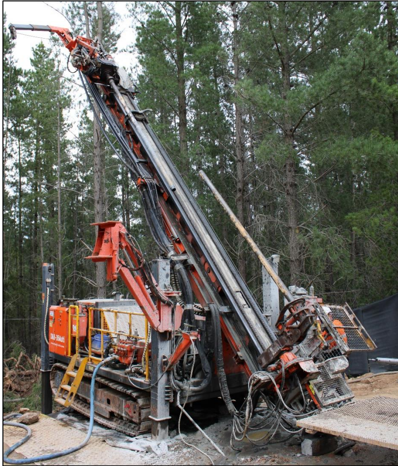
Figure 2: Diamond drill rig in operation at the Lightning Prospect, Castlemaine Gold Project (EL006679)
