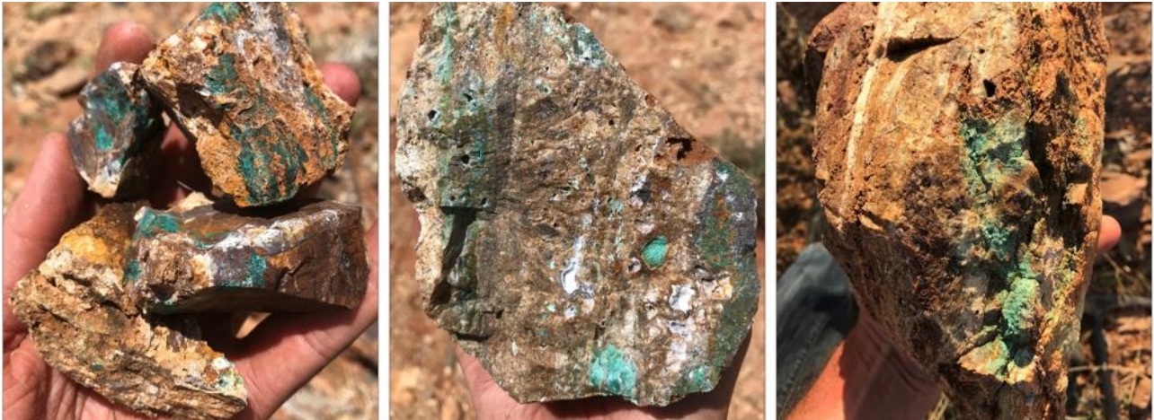
Figure 6: Examples of Ningaloo mineralisation. ABOVE LEFT: Sample JE0074 malachite-azurite with quartz and Fe-oxides with 3.92% Cu; ABOVE MIDDLE: Sample JE0075 malachite-azurite with quartz and Fe-oxides with 2.47% Cu + 2.71g/t Ag; ABOVE RIGHT: Sample JE0045 malachite-azurite with quartz with 10.3% Cu + 3.8g/t Ag.
