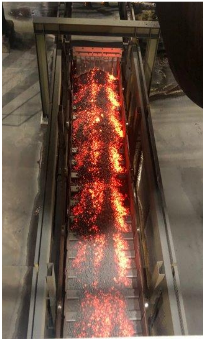
Steel Pan Conveyor transporting hot pellets
