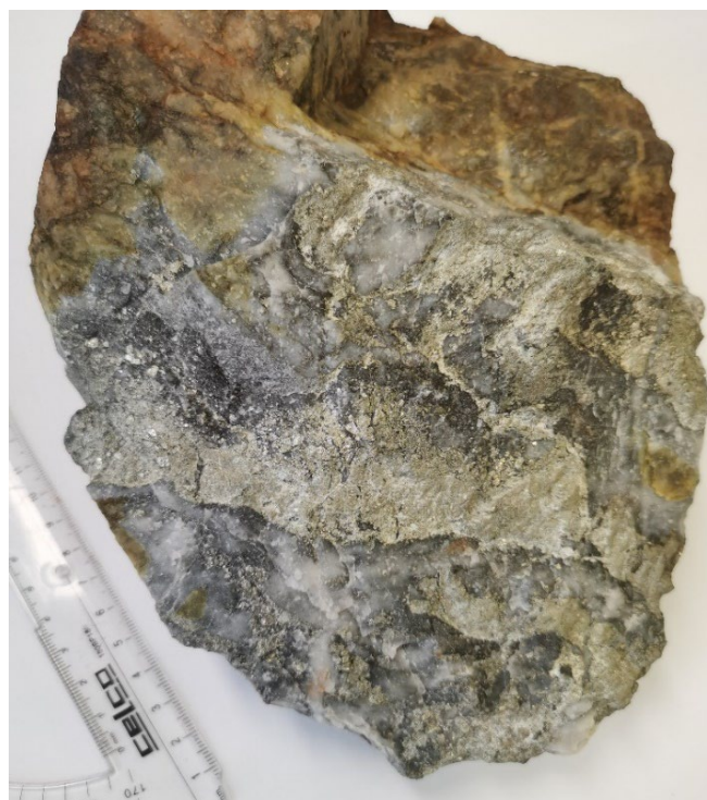
Figure 5. Rock recovered from the Lord Henry waste dump, showing high-grade mineralisation containing significant sulphide material
