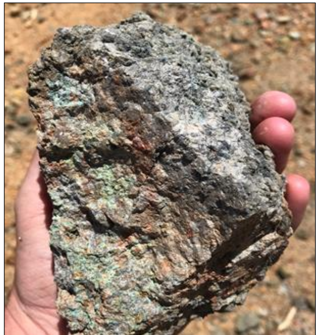
Figure 3 RIGHT: Hand specimen of material that was subsequently found to contain 1,165g/t silver, 0.26g/t gold and 0.35% copper (rockchip sample number MC0025). This result and photo were first reported in Inca's ASX announcement dated 4 October 2019.
