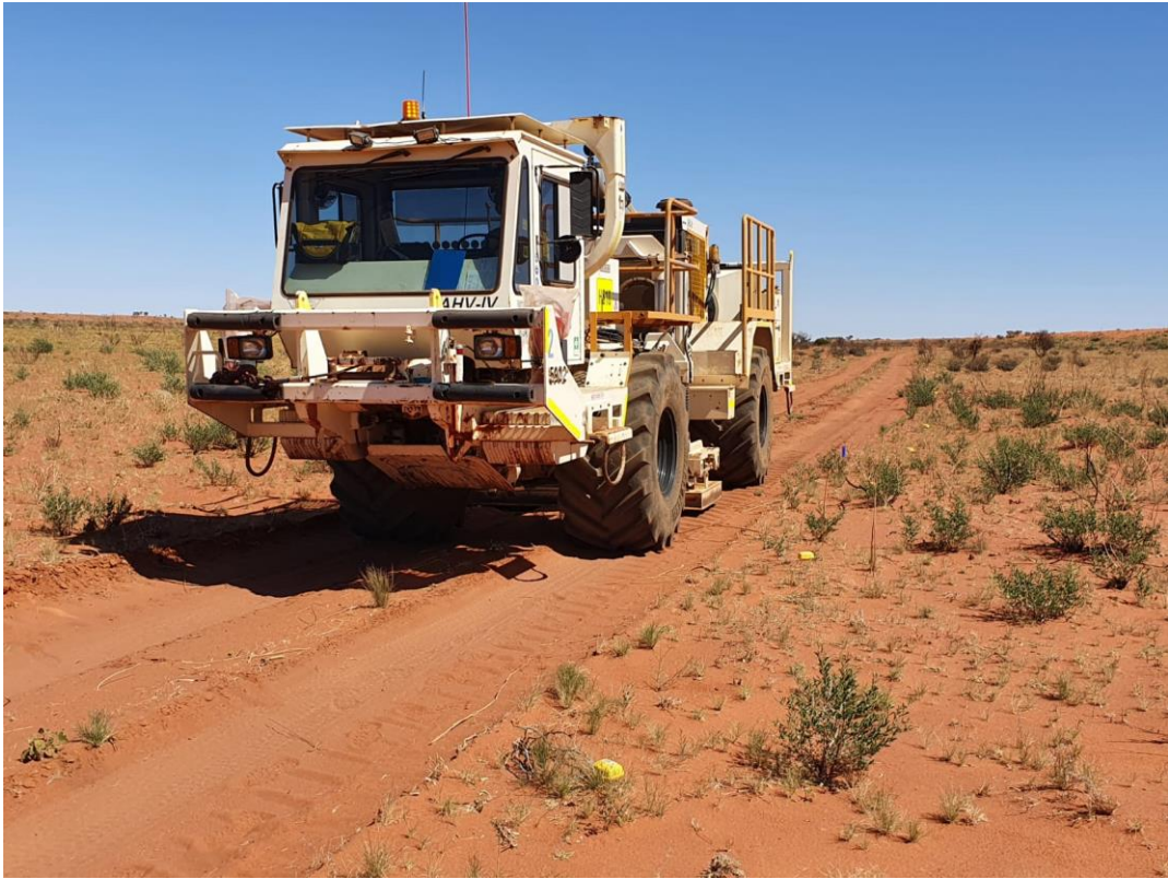
Figure 3 Hiseis Inova AHV-1V 62,000lb seismic vibrator truck with Inova Quantum receiver nodes layed every 5m along the track
