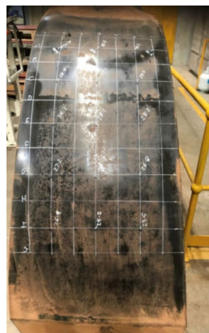
Fig.2c): ArmourGRAPH™ Liner After 62 weeks.
