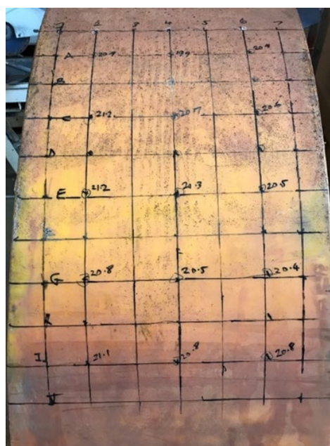
Fig.2b): Standard PU Liner After 62 Weeks
