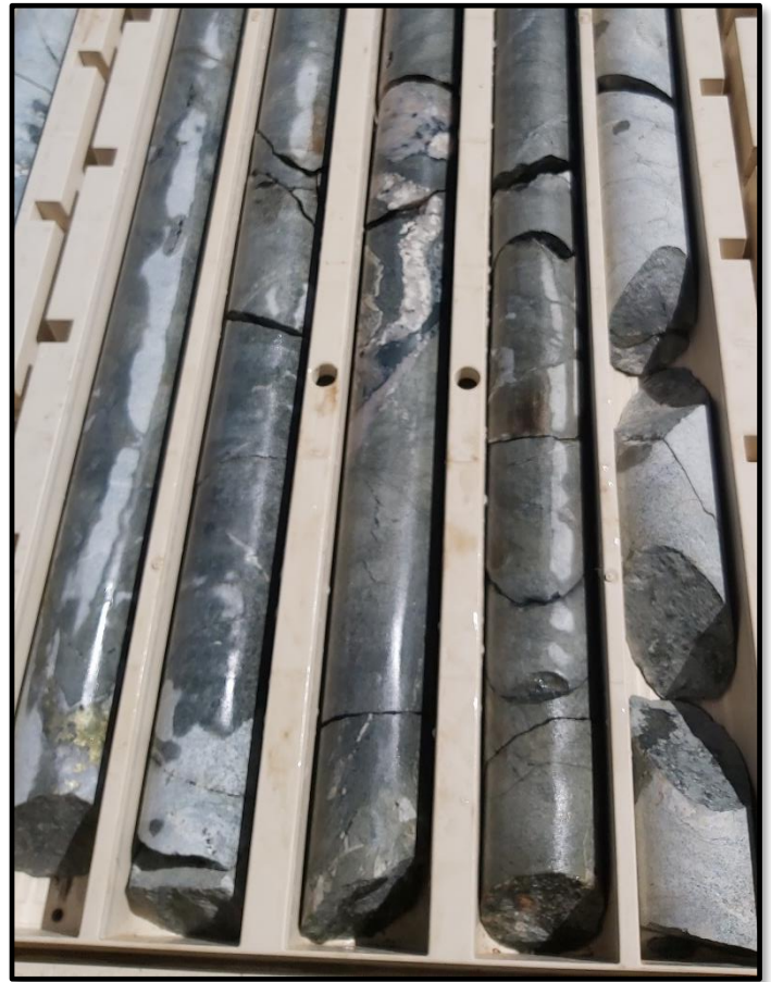
Figure 1 – AWN002 drill core with quartz veining and pyritic, chalcopyritic massive veining in chloritic-phyllic altered host
