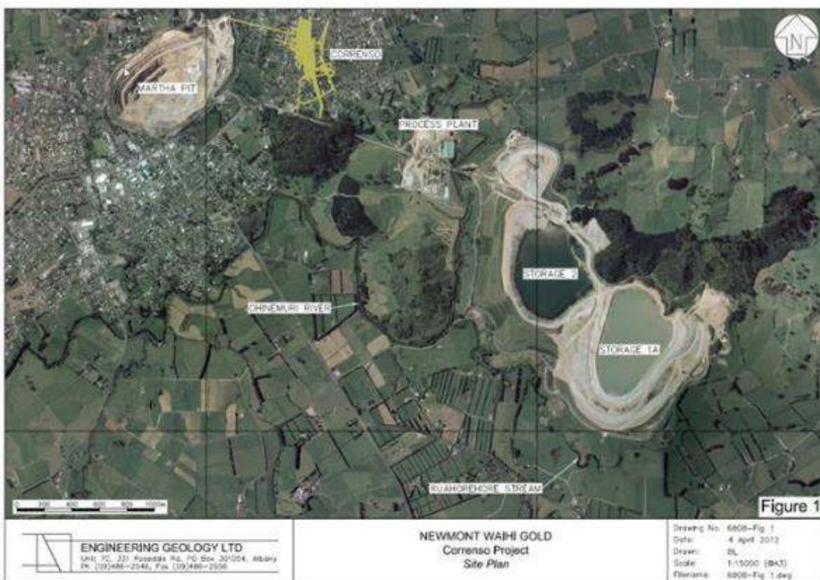
Figure 18-2: Location of Tailings Storage Facilities
