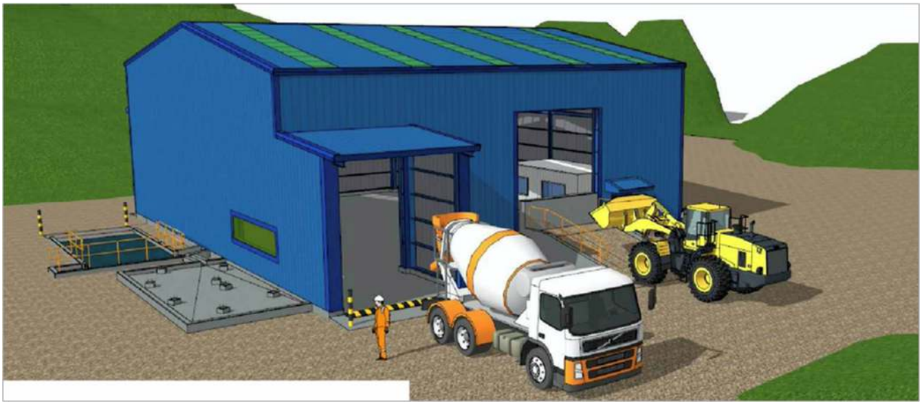
Figure 16-27: Dry Mix Cement Backfill Plant
