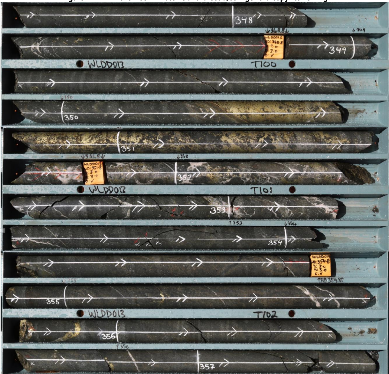
Figure 1 – WLDD013 – semi-massive and breccia/stringer chalcopyrite veining
