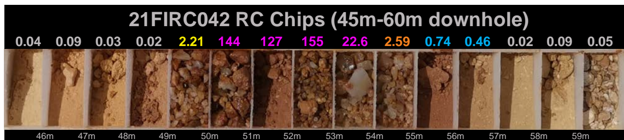
Figure 2. RC chips of significant intercept of 6m @ 75.57 g/t Au from 49m downhole in hole 21FIRC042.
