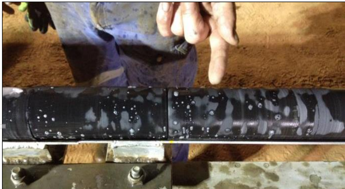
Bleeding gas was seen from all carbonaceous intervals within M. Velkerri Shale: Tarlee-S3
