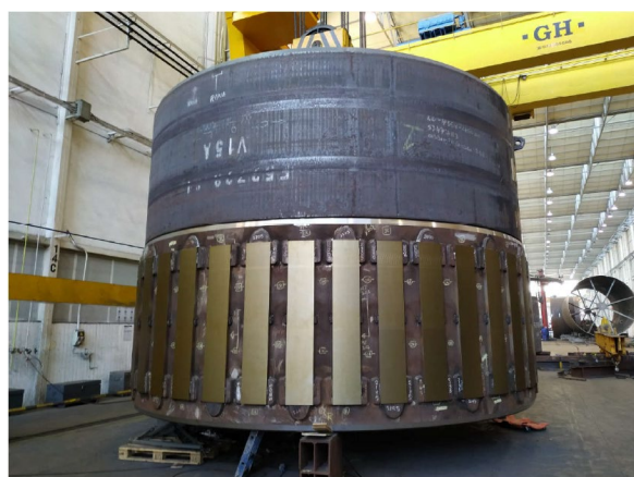
Kiln tyre shell section with supporting blocks
