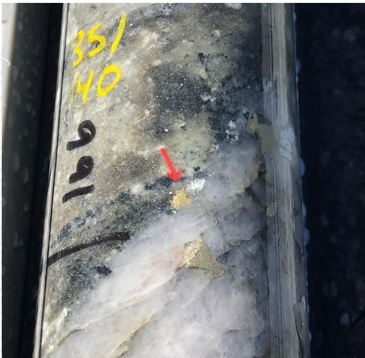
Image 5 – Visible gold in MDGT004 from 166.0m
