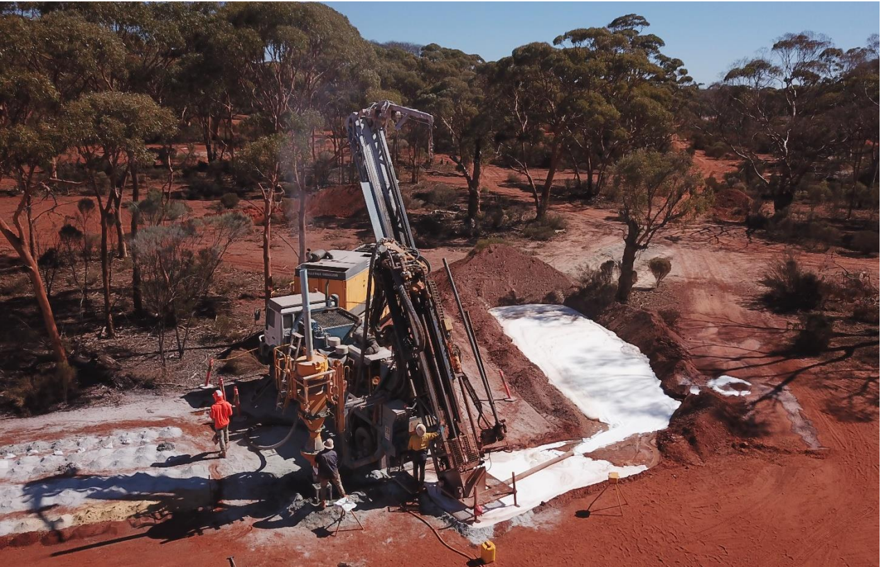
Image 3 - RC drilling at Mandilla East
