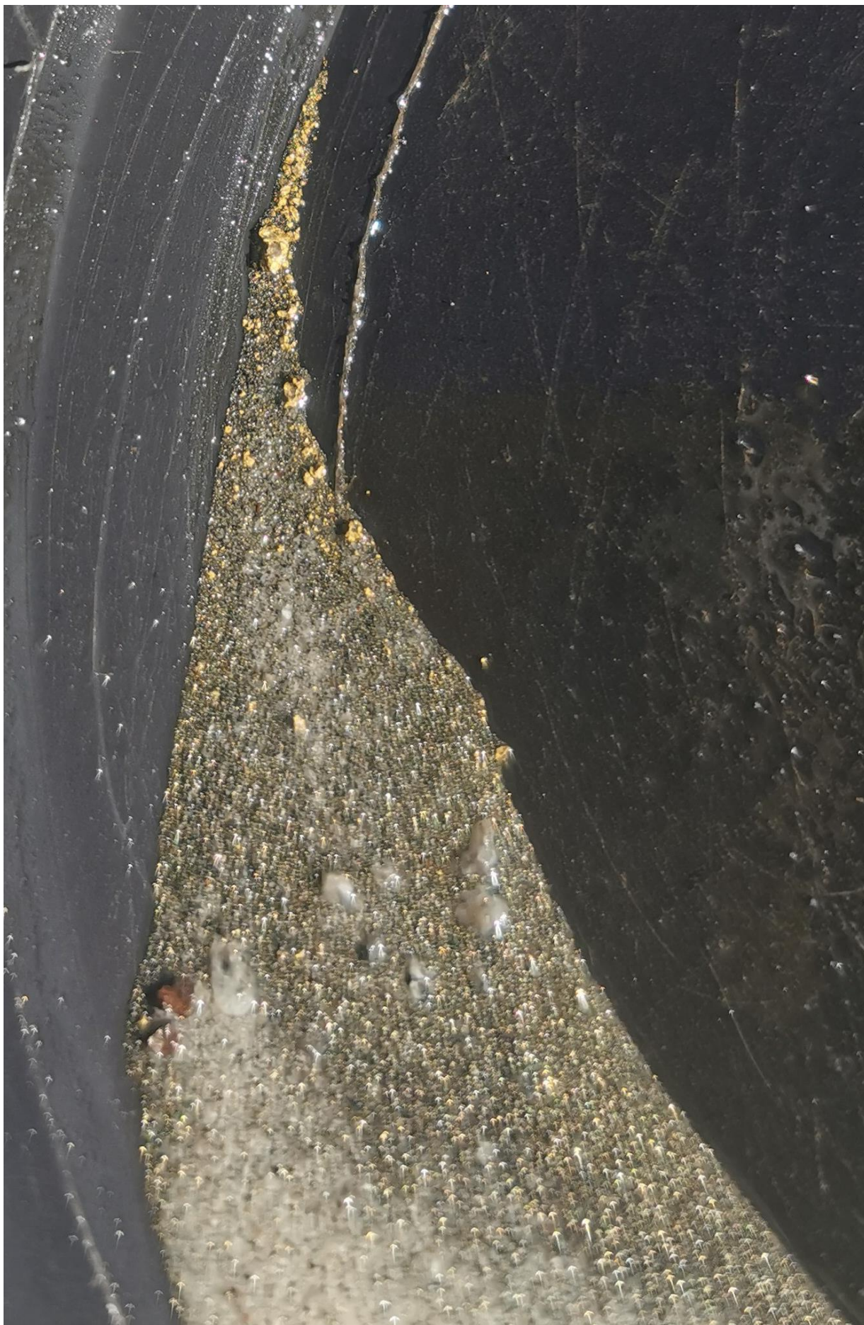
Image 2 - Visible gold in MDRC324 from 102m - 103m
