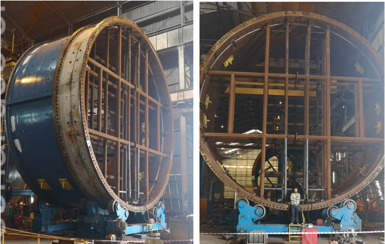
Figure 3: SAG mill shell undergoing refurbishment.
