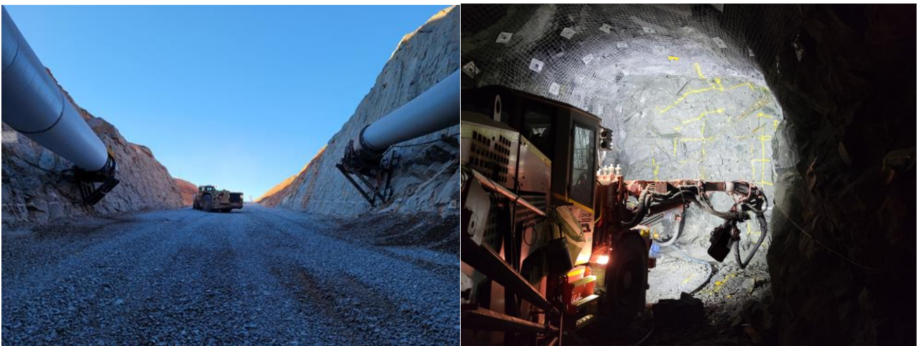
Woodall Decline (L to R) – Bogger leaving Box-cut and Jumbo boring face
