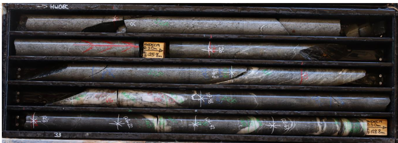
Figure 9: Resource Definition drill core from HWDEC019 (0.6m @ 168g/t Au) showing andesite and porphyry-hosted quartz veining, shearing and alteration with coarse visible gold. Lode intersection is located 20m past the limits of the current Mineral Resource wireframe.
