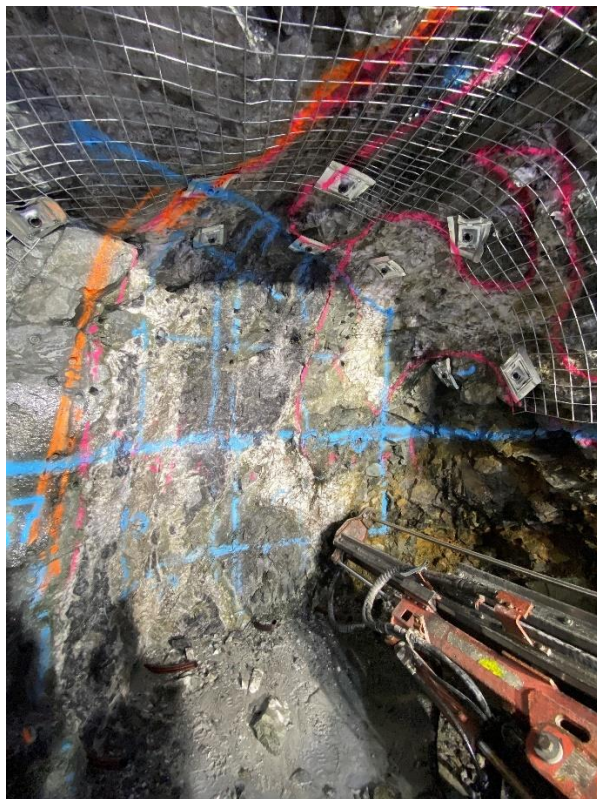
Figure 4: Rothsay development ore drive face (vein grade 31.6 g/t with average face grade 17.6 g/t)
