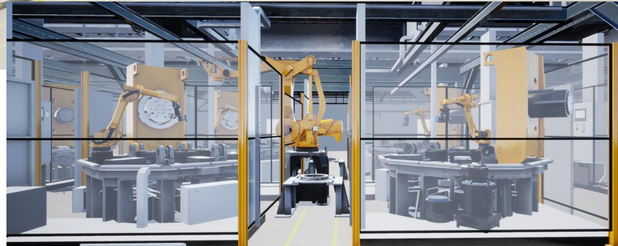
Multiple Generation 2 Moulding Stations in Mega-line with robot vehicle loading capability 1
