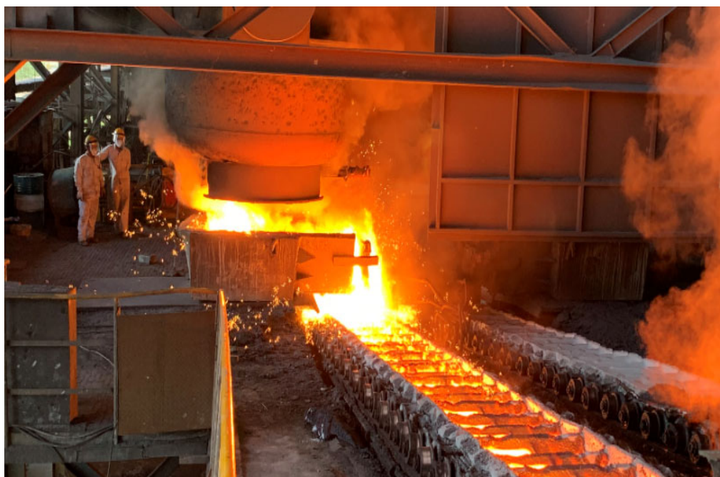
Ingot casting of NPI
