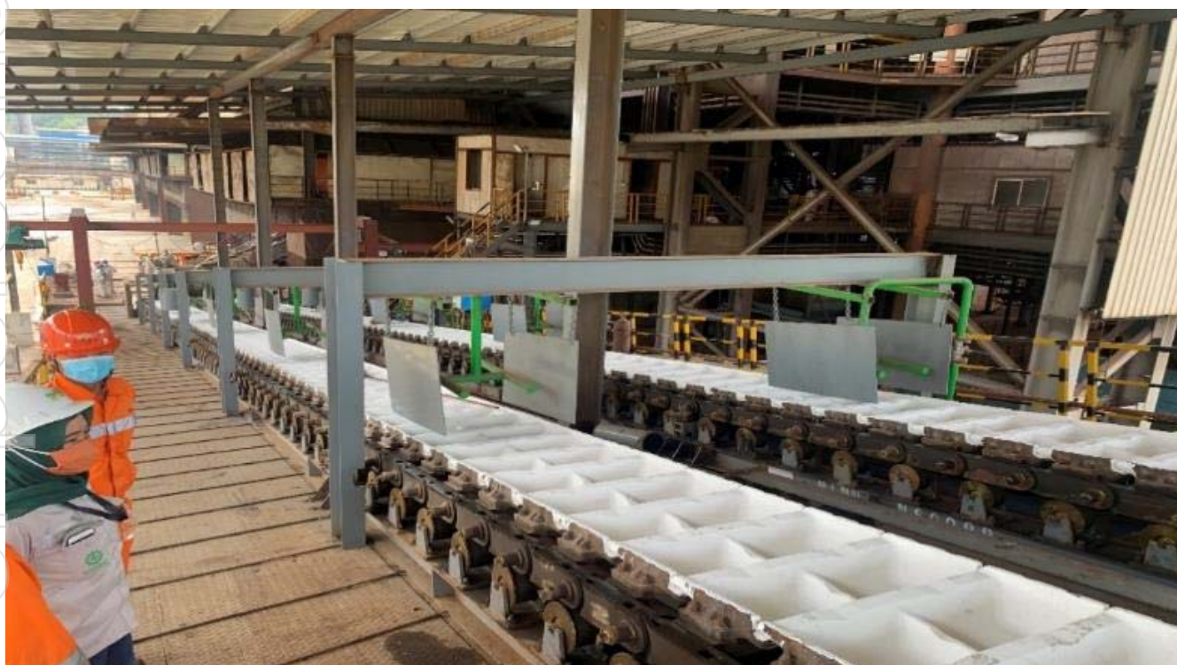
Commissioning of ingot conveyer at Ranger Nickel
