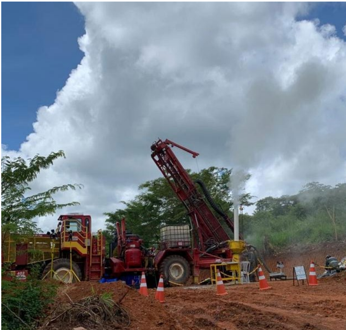
Figure 1 – Geosedna RC rig drilling first hole at the Leão Prospect
