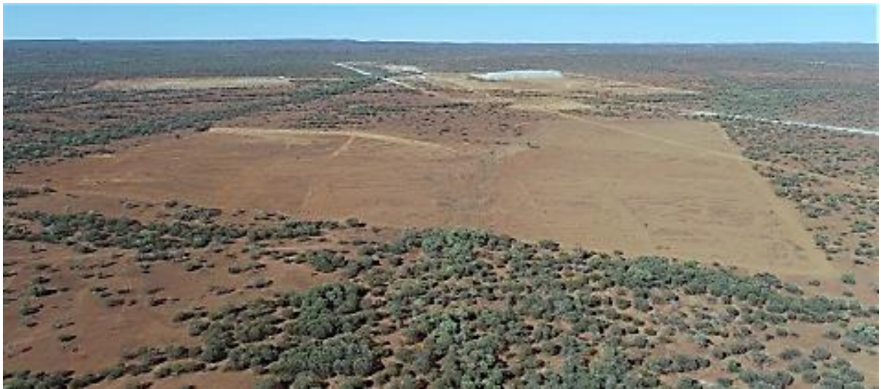
Figure 2. Aerial view of topsoil strip of TSF.
