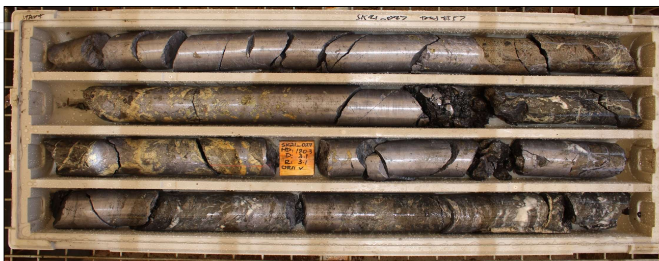
Figure 9: Drill core from hole SK21_027 massive galena showing part of the intersection of 9.5m @ 45.5% Pb, 4.1% Zn, 425g/t Ag from 174.4m
