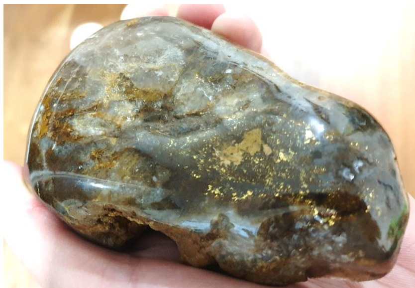
Photo 1: Photograph of polished gossanous quartz vein with abundant visible gold recently sampled by Silver City from the outcrop exposures in the north face of the Brians historic pit.
