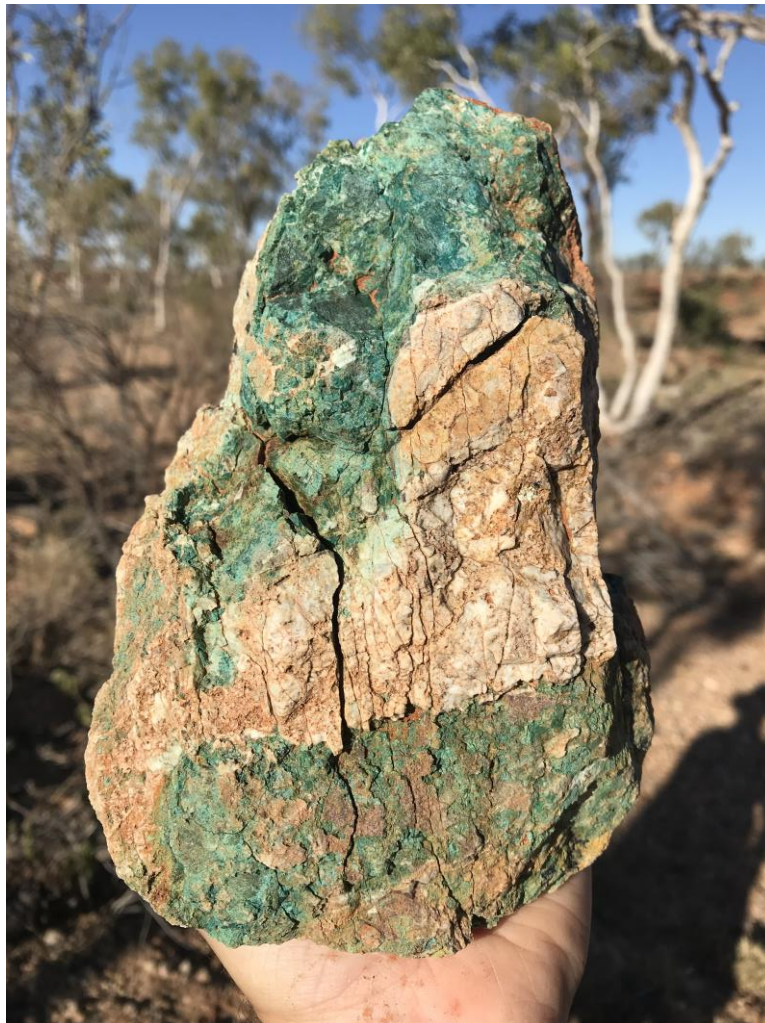
Figure 5. Photo of rock chip sample JE0107 collected at the location of a new Cu-Qtz-Fe vein at Ningaloo (Figure 3 for location). The sample comprises massive malachite and thin quartz veins in what was originally a granite.
