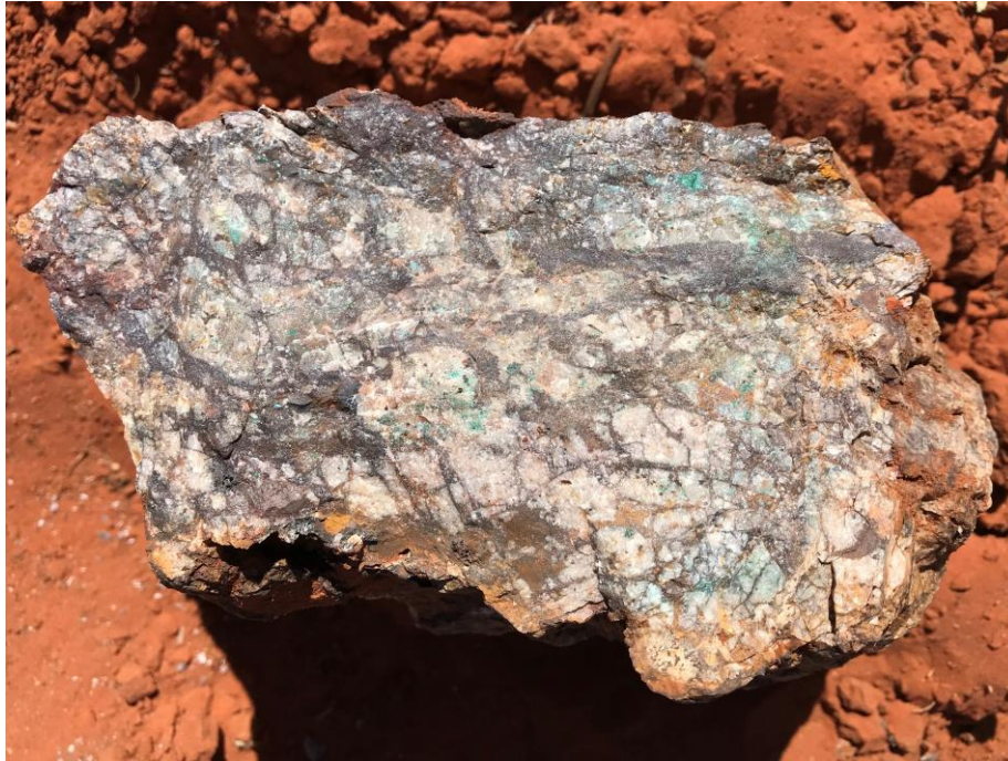
Figure 4. Photo of rock chip sample JE0101 collected at Ningaloo (Figure 3 for location). It is quartz-haematite breccia, the quartz forms the clasts (white) and the haematite from the matrix (red-brown). Disseminated chalcocopyrite and malachite occurs in the matrix. This one sample reveals two phases of hydrothermal activity, a first phase of milky white quartz and a second phase of haematite-copper.
