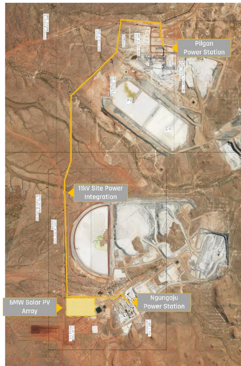
Pilgan and Ngungaju facilities interconnection and solar PV array
