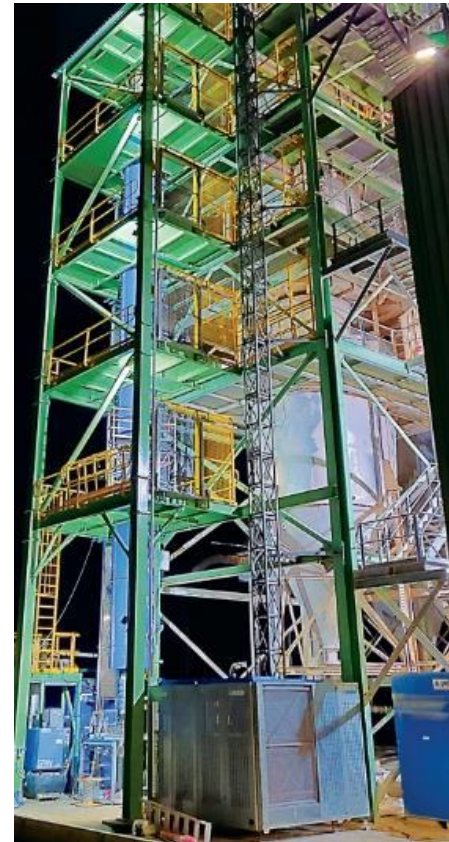
Left: Calix BATMn electric vertical reactor kiln enabling renewable energy powered calcination
