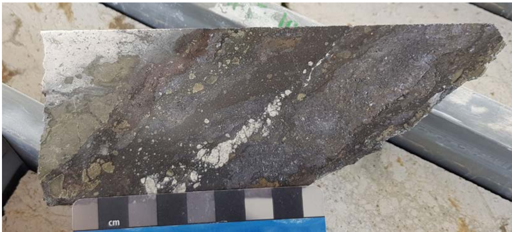
Figure 2. 128.1 metres in BD21002 (Main Zone) - Northern Feeder vein, with 1 metre @ 1,490 g/t silver, 4.36% lead and 2.2% zinc. Includes massive sulphide of sphalerite, galena and silver sulphides.
