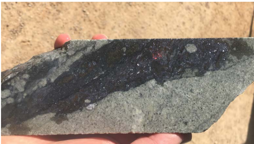
Figure 3. 279.4 metres in BD21001 - Northern Feeder vein, with 1 metre @ 1,290 g/t silver, 4.10% lead and 2.06% zinc. Includes massive sulphide of sphalerite, galena and silver sulphides.
