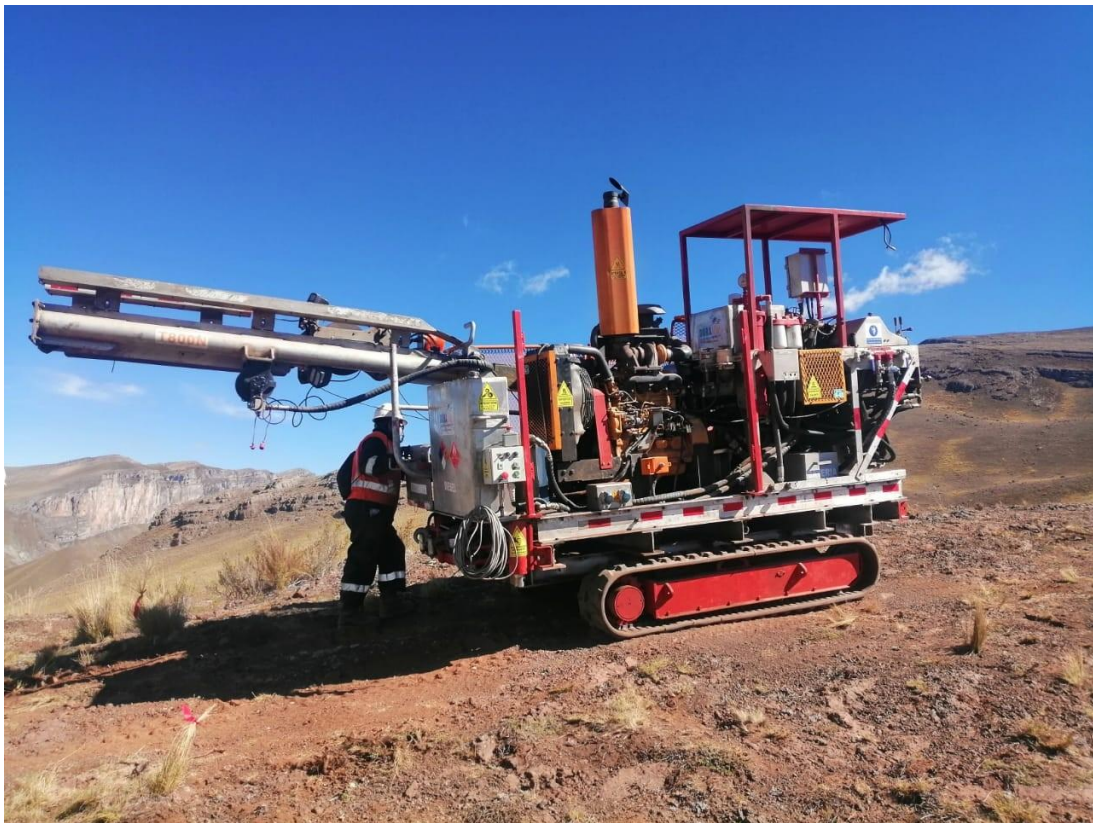
Photo 3: The drill rig whilst mobilising to the platform. As a highly manoeuvrable track-mounted rig, elaborate access tracks were not, and will not be required for most of the NE Area FTA drill program. Notwithstanding the compactness of the rig, diamond core drilling can reach depths of greater than 1,000m. The deepest hole in our program is 750m.
