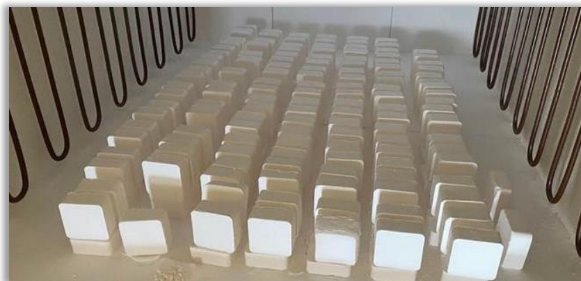
Sintering of HPA pellets for sapphire glass manufacture
