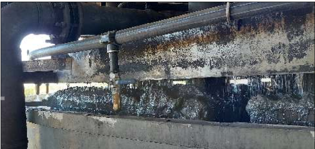
Figure 1: Jameson Cell commissioning, with production of saleable concentrate directly from the Jameson Cell at the Century Zinc Mine
