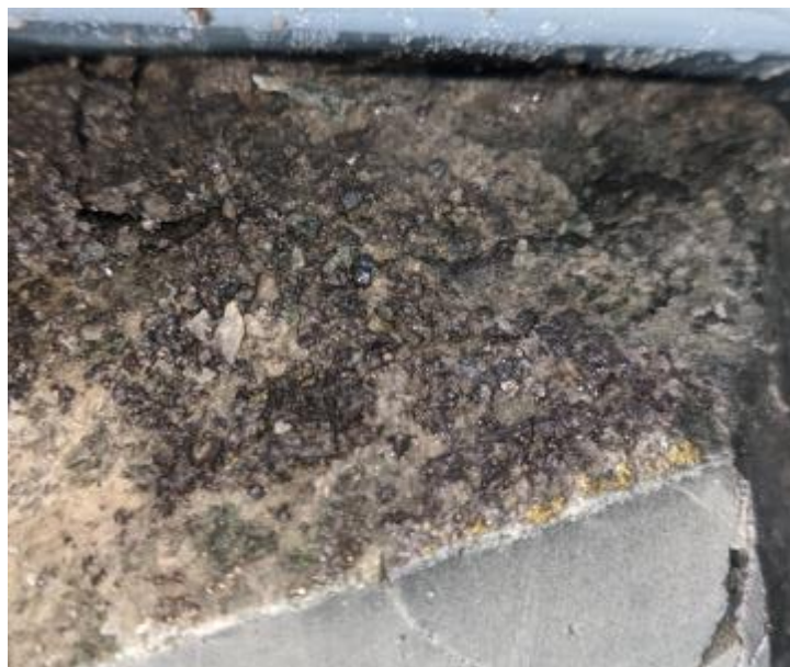
Chalcocite coating of pyrite at 66.1m.
