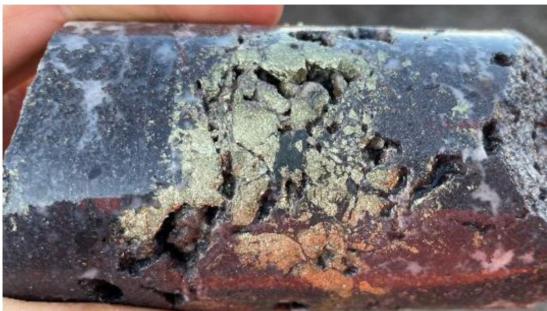
Vuggy chalcopyrite-clast breccia in massive hematite+quartz. 539.2m.
