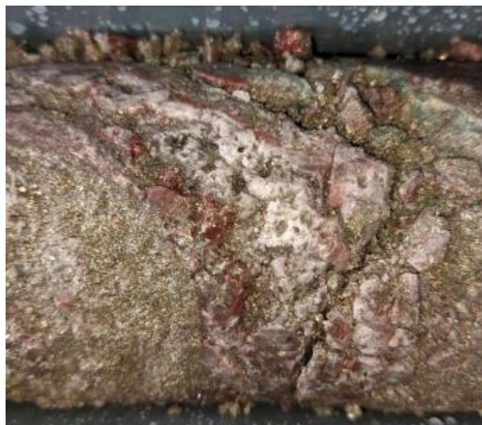
Quartz hematite pyrite vein in lode at 349.2m.
