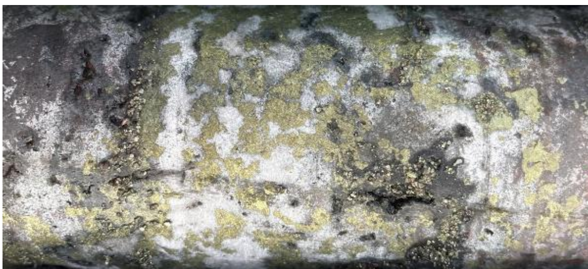
Intergrowth of chalcopyrite+quartz/carbonate, partly replacing massive hematite with laths of hematite. 553m.
