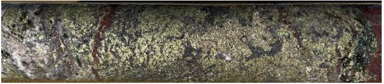
Massive chalcopyrite+pyrite. Dips moderately toward the NNW. 529.6-530.1m.
