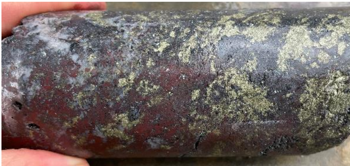
Semi-massive chalcopryite+pyrite in hematite+magnetite+quartz rock. 476.7m.
