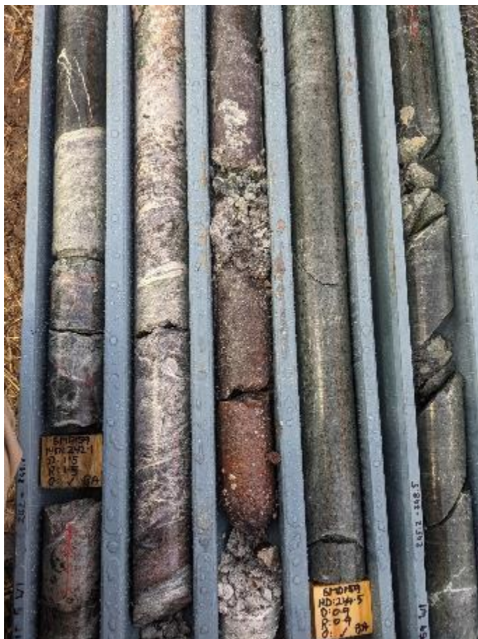
Hematite alteration in position of Cayley Lode at 244m.
