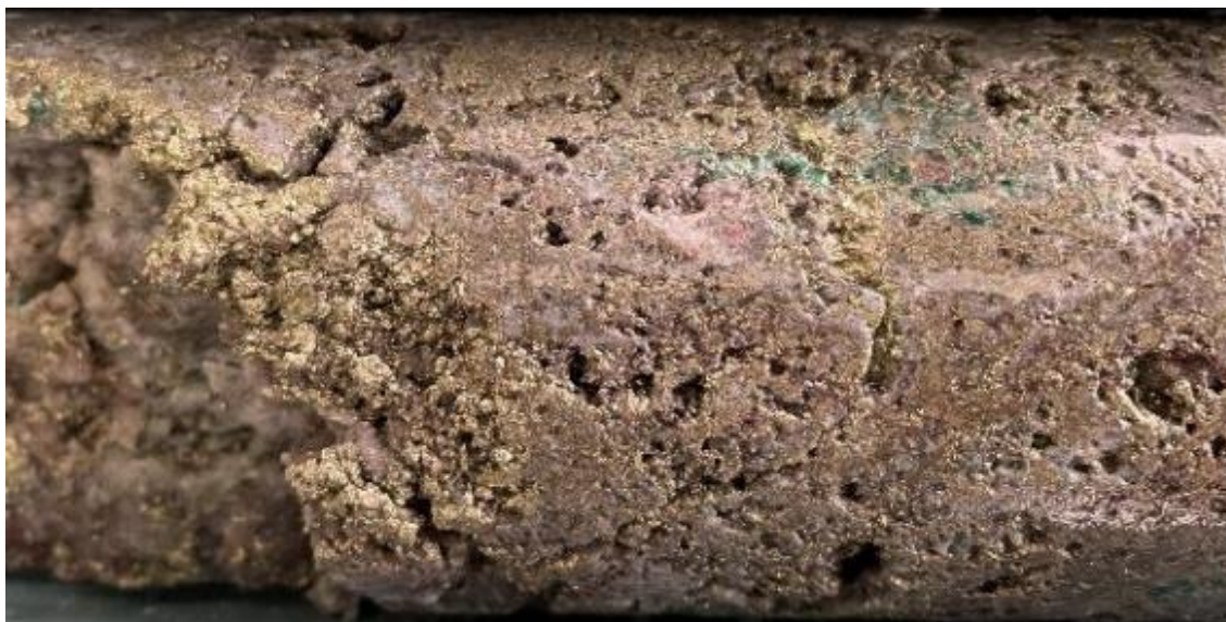
Disseminated and semi-massive chalcopyrite+pyrite in vuggy quartz rock. Trace fuchsite. 478.5m.
