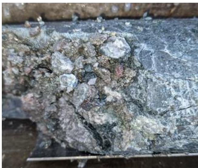
Trace pyrite hematite veining at 600.5m.
