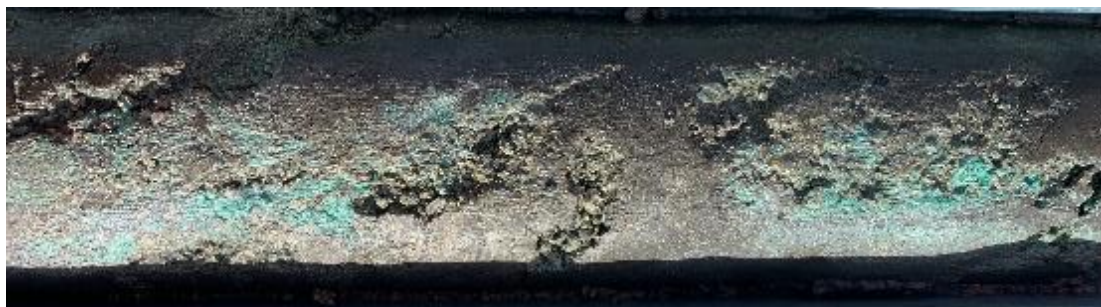
Pyrite-chalcopryite-fuchsite lode at 475.2m.
