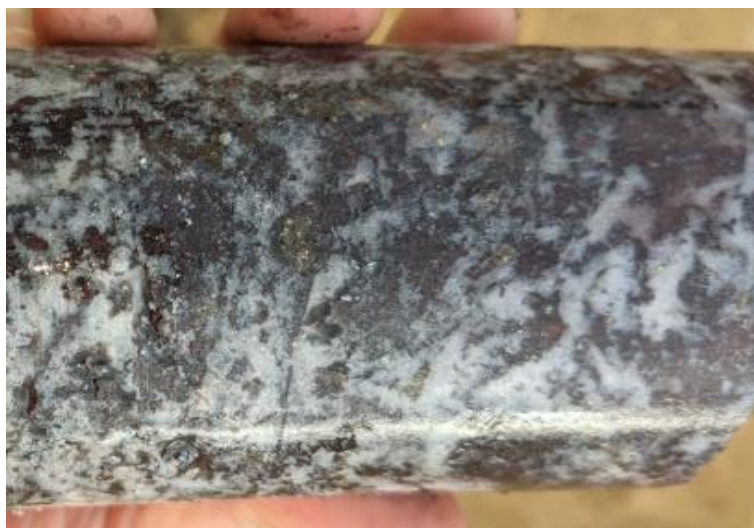
Hematite quartz chalcopyrite veining at 418.6m.
