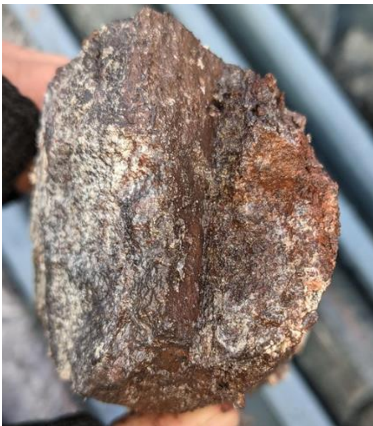
Strong hematite altered serpentinite just above the LAS at 244m.
