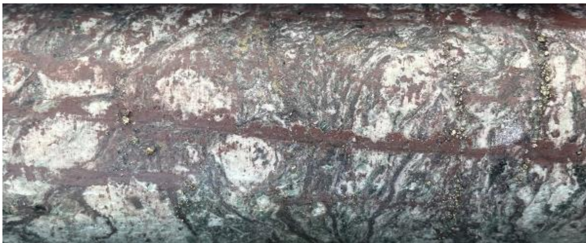
Clay+hematite-altered ?serpentinite. 553.4m.
