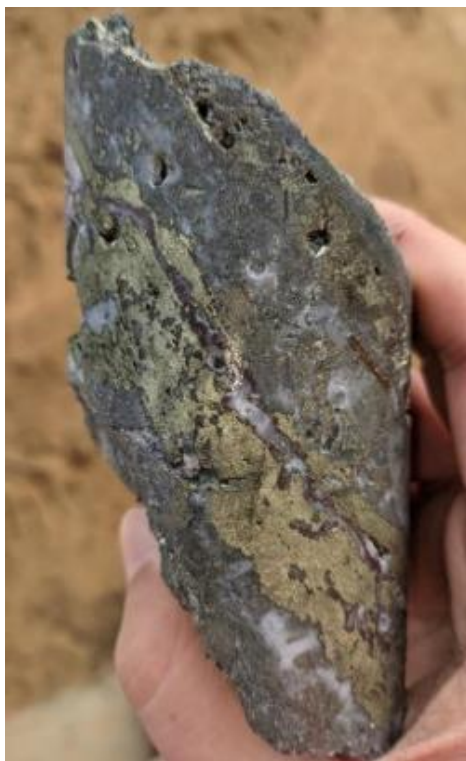
Quartz chalcopyrite hematite veining at 350.3m.
