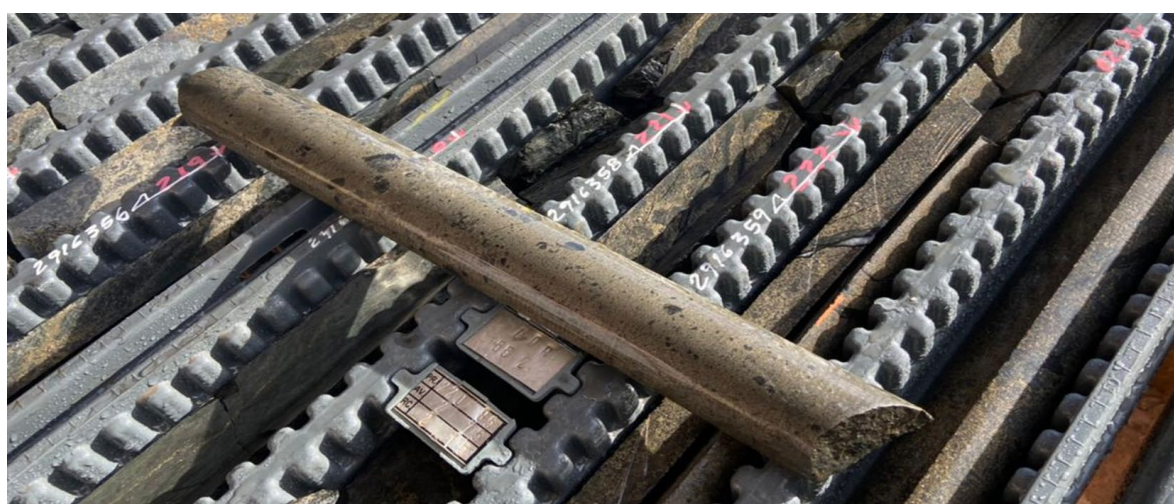
Figure 1 – Core from drill hole JAG-DD-21-151 (Jaguar South); Semi-massive and massive sulphides (metallic bronze/yellow colour), predominantly pyrite, millerite and pentlandite, hosted in an altered dacite.
