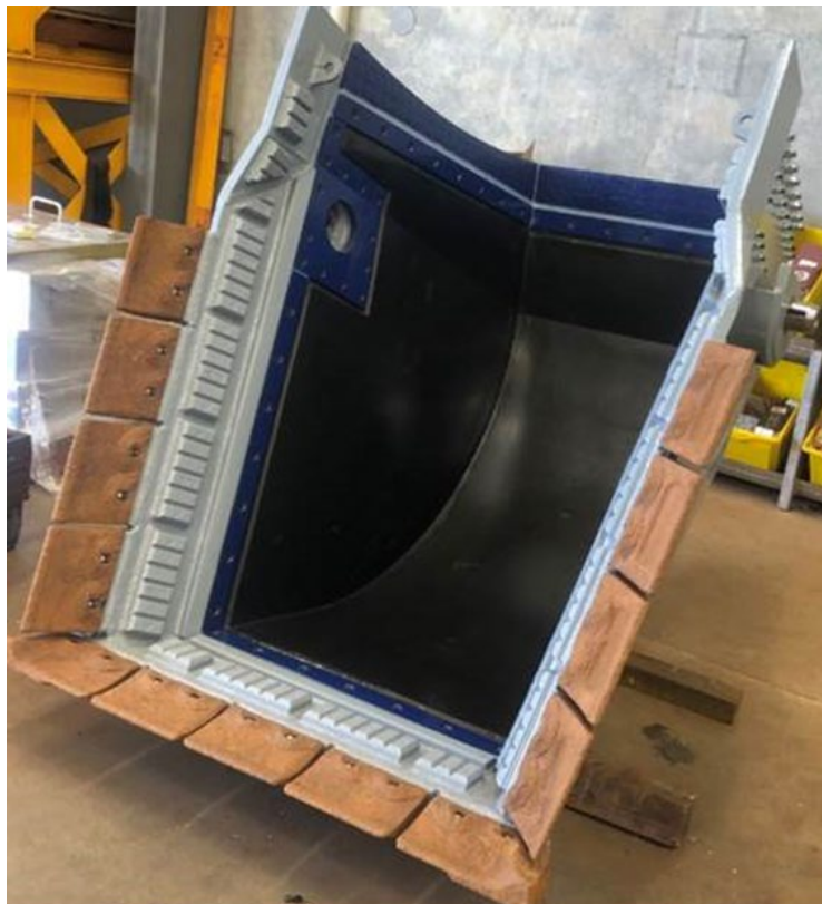
Figure 4 - The newGen Group ArmourGRAPH Bucket Reclaimer wear liner.
