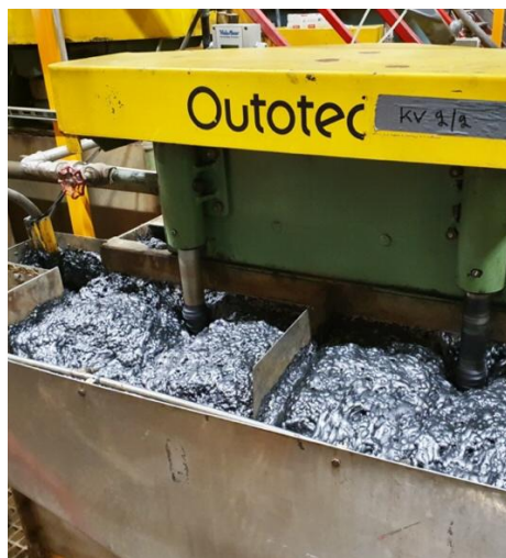
Figure 9 60 tonne bulk sample of Vittangi graphite ore being milled and concentrated at GTK, Finland.
