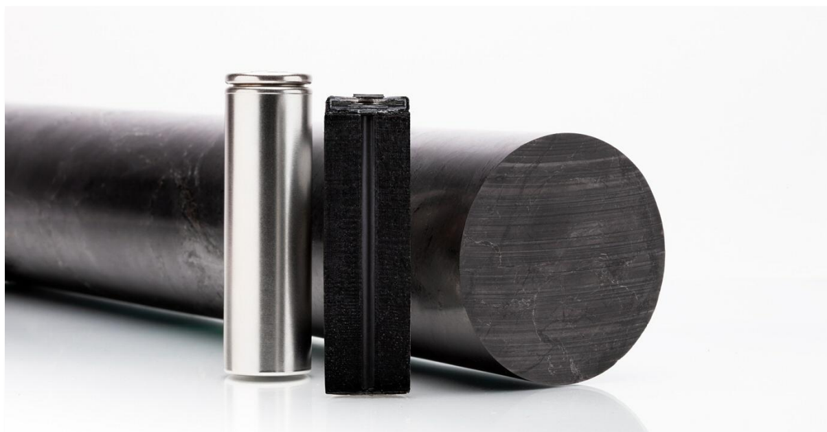
Figure 20 Vittangi graphite drillcore and commercial cylindrical Li-ion battery showing the internal structure and graphite anode layers.
