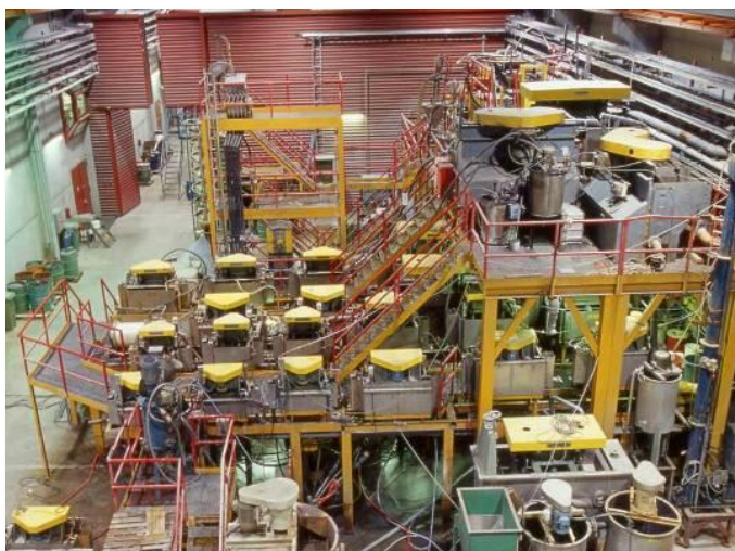
Figure 9 60 tonne bulk sample of Vittangi graphite ore being milled and concentrated at GTK, Finland.
