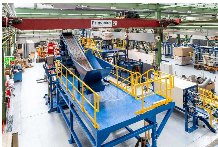
Figure 1 – Two stage Shredding Circuit
