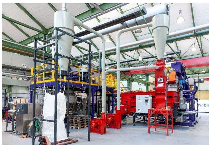
Figure 6 –Shredder feeding into – Primary Classification Circuit (foreground -red) removes and bags plastics and Cu/Al metal foils
