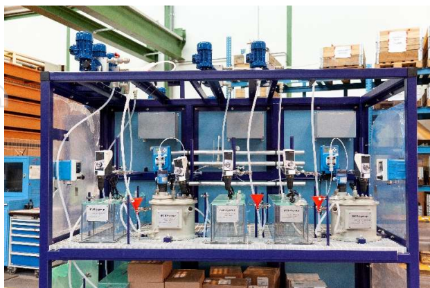
Figure 9 – Single Solvent Extraction Mixer/Settler Circuit
