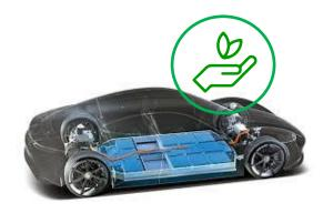
The key battery cathode material in EVs, high nickel NMC 811 batteries are the favoured chemistry
